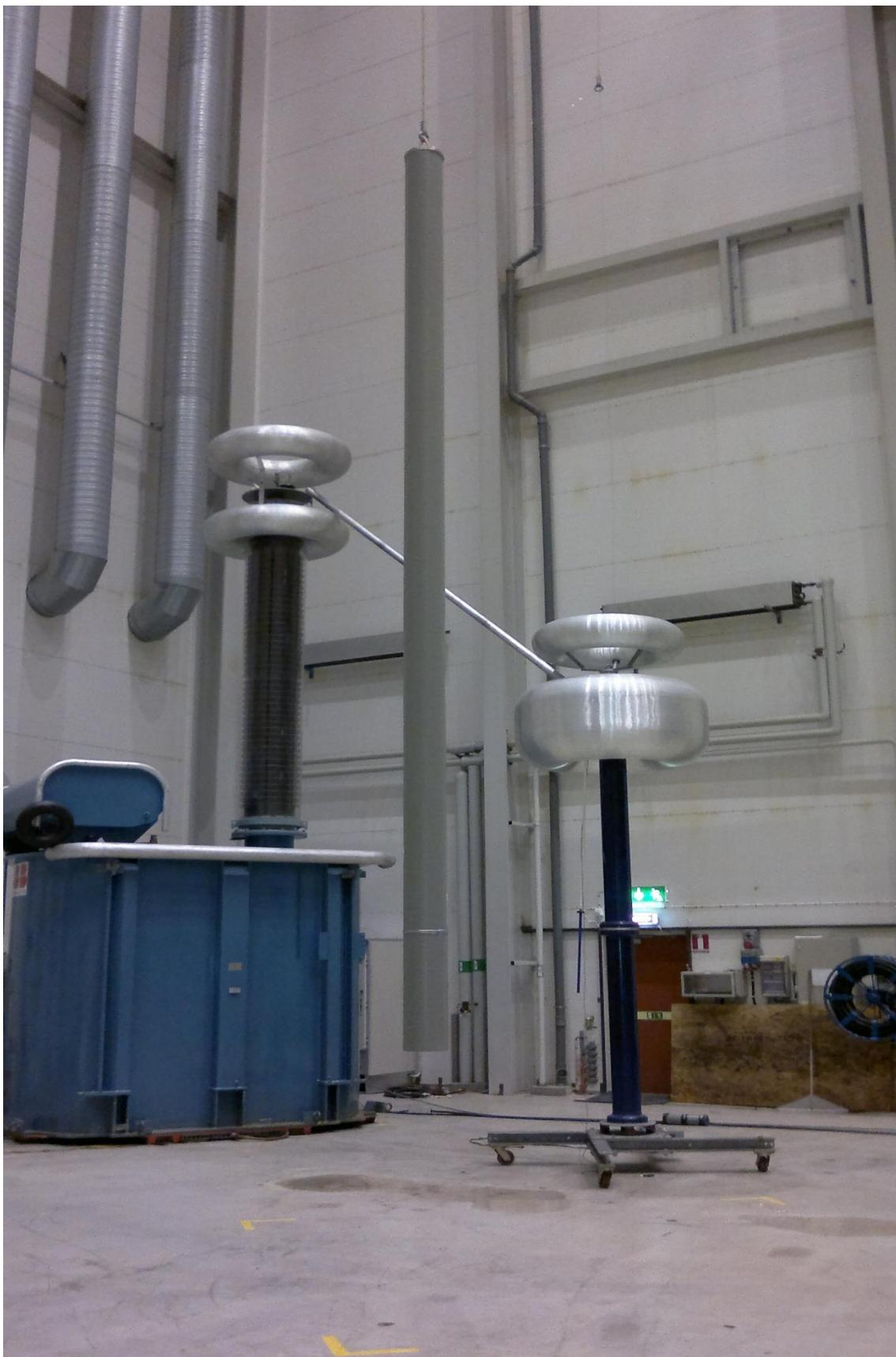
Dry AC withstand test of one 600 mm section
